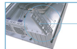
Easy assembly for add-on cards
